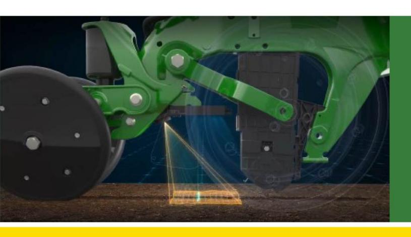
FurrowVision gives operators real-time video of the open section of furrow between the Tru-Vee openers and closing system.
